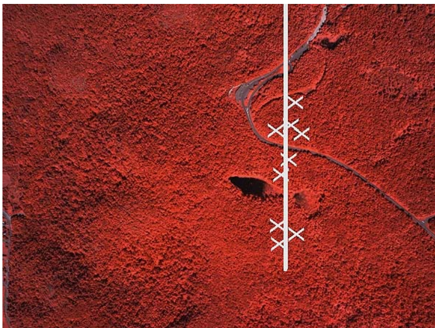
Figure 2. CIR composite image showing some of the plots in a study of temperate hardwood forest damage assessment following a severe ice storm. The image was acquired with a Kodak DCS CIR 460 digital camera. Pixel size is 57 cm.
